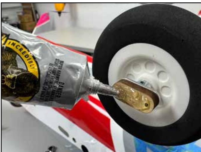
Install the wheel pant over the wheel and axle, tighten to the landing gear with screws as shown, using blue loctite. The wheel pant support should sit against the pant as shown. By stabilizing the pant, this design lengthens the life of your wheels pants. Just like on full-size aerobatic aircraft, however, wheel pants take a lot of abuse and over its life your aircraft will probably need a replacement set.
