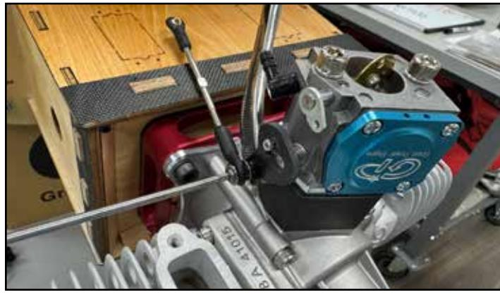
The 88" Extra 260 uses a full-size throttle servo with a 1" arm. There are two generic throttle servo locations provided, one for right-hand and one for left-hand carburetors. To get the best linkage geometry with our install, we elected to use the plywood servo mount pieces included in the kit and custom-mount the servo as shown.
