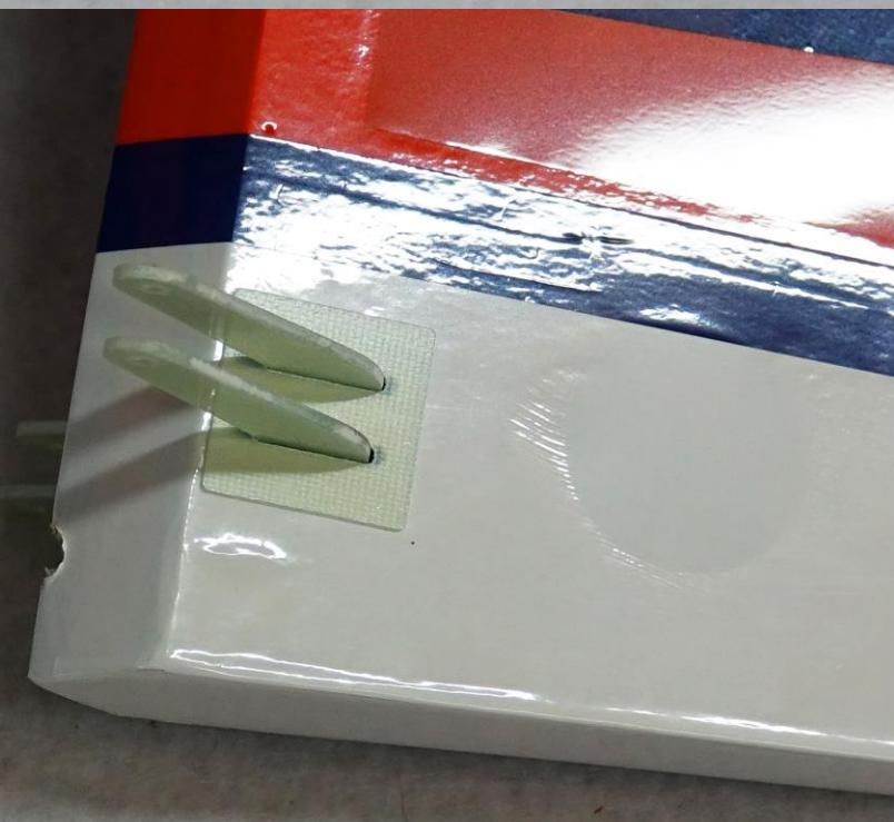
**13. Locate a 2mm ball link from the hardware bag. Drill a hole 2 inches back from the leading edge of the rudder on the bottom of the rudder surface to accept the shank on the ball link.**
