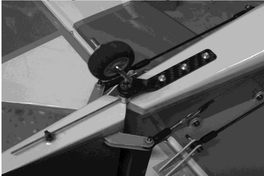
**15. Position the tailwheel assembly on the rear bottom of the fuselage and be sure the tailwheel wire is aligned with the rudder hinge line. Secure the tailwheel with a couple of pieces of masking tape while you drill 2 holes with a 1/16" drill bit. Apply a few drops of thin CA to the holes and allow to dry then secure the assembly to the bottom of the fuselage as shown with the 2 provided wood screws.**
