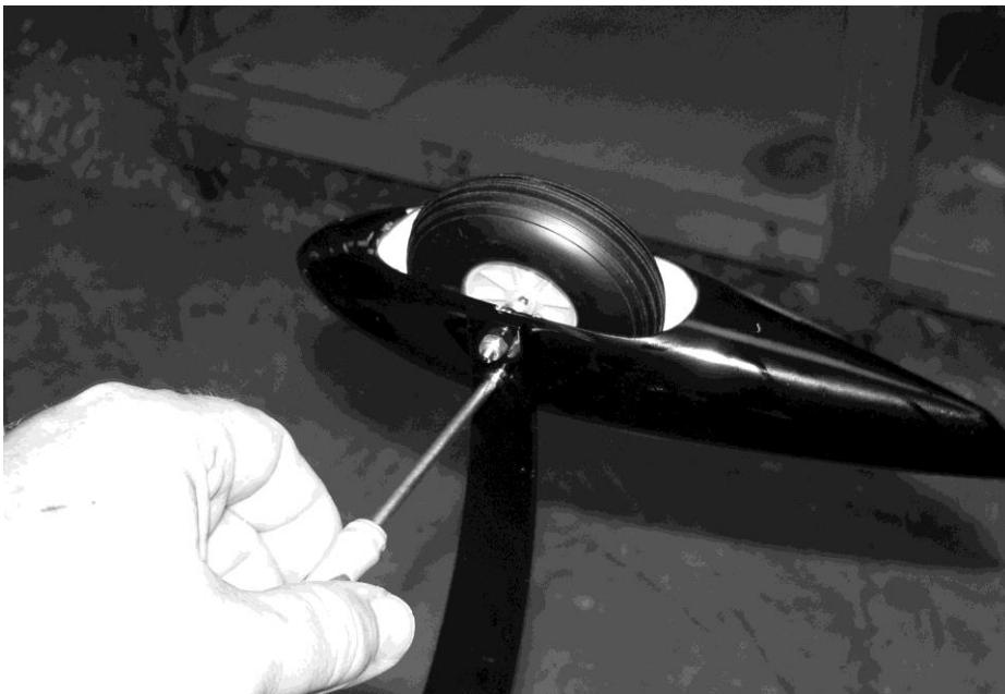
**20. While the Extra is still upside down let's install the rudder and finish up the tailwheel installation. Apply 30 minute epoxy to the holes in the rudder post and to the rudder hinges. As you position the rudder onto the vertical fin, be sure the tailwheel tiller arm is inserted into the ball link. Push the rudder into position and wipe away any excess epoxy with a paper towel and denatured alcohol.**
