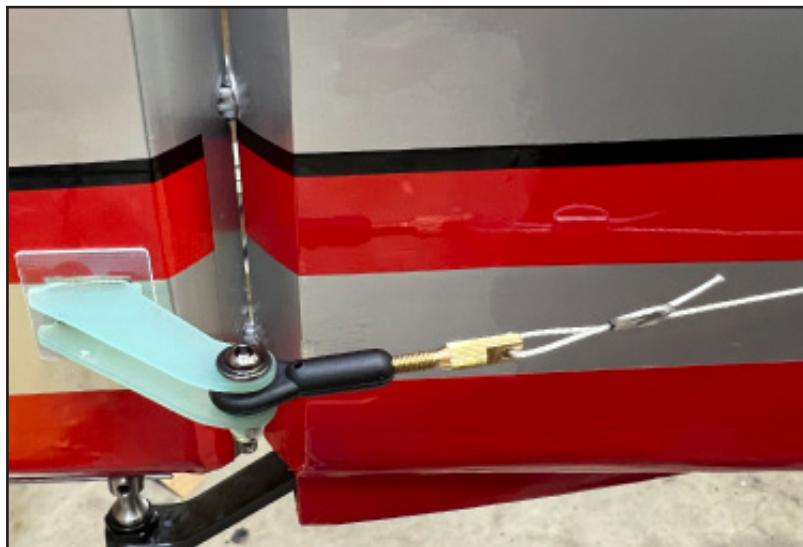
The pull-pull rudder setup is the best choice for all typical power systems, but if you decide to use the rear-mounted push-pull system, begin by locating the rudder servo mount on the **RIGHT** side of the fuselage as shown. The mount is recessed into the fuselage. NOTE: the mount is recessed and, for some servo/arm combinations, you will need to space the servo up from the mount. On this installation of SAVOX 1270 and EF arm, we used approx 2mm of spacers under the forward servo mount pads.
