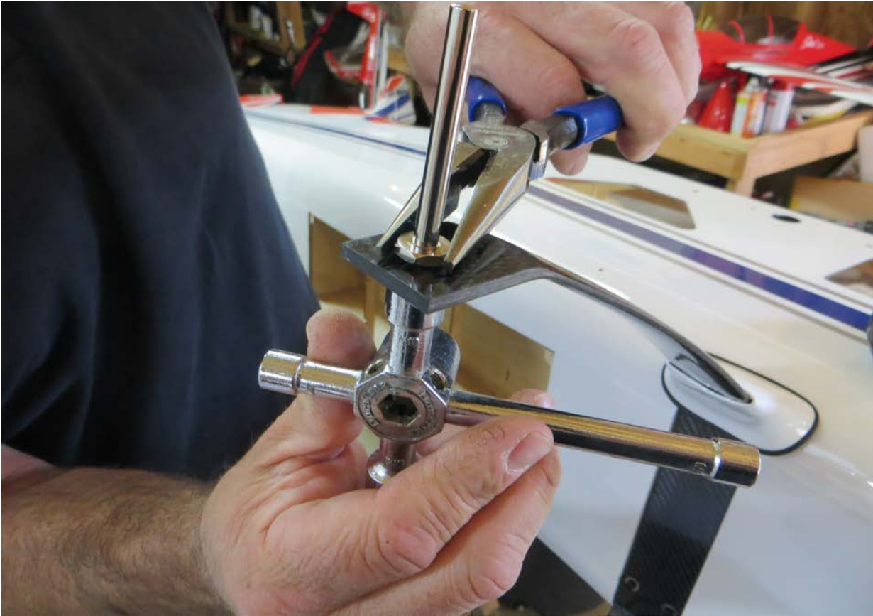
18. Attach the axles to the carbon gear with the supplied washer and locknut.
