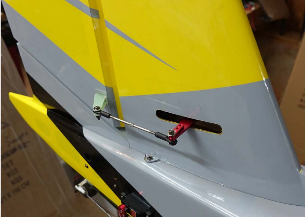
36. Slide the carbon fiber rudder mounting tube into the receptacle in the fuselage. Slide the rudder into position and secure with 2 3mm bolts and washers.
