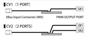
\* This product converts the XBus signal to a PWM signal that then allows the use of normal/PWM (non XBus) servos with JR/DAF's XBUS system. \* This product does not have an integrated regulator. Please check the rated voltage of the target products and use the proper source battery for the receiver. \* Channel (ID) setting for each output connector must be performed by either the XBUS Channel Programmer or wirelessly from a JR/DFA transmitter fitted with XBus.
