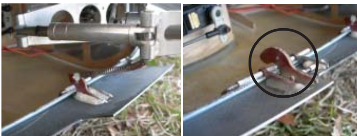
Close-locks for front and rear door and connection pin between both doors
