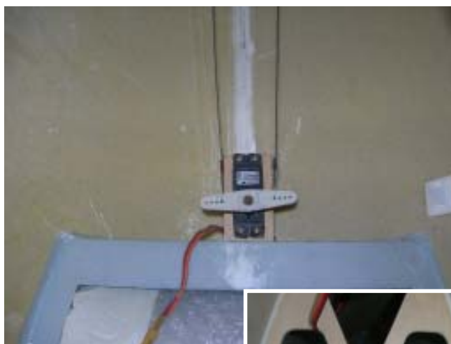
Position of tail gear steering servo and location for the pull/pull wires to the tail gear control horn.
