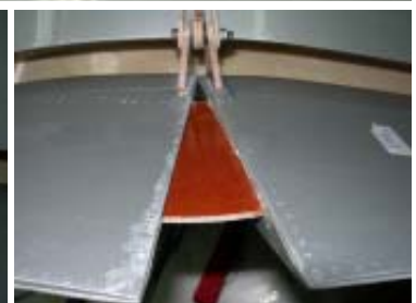
Allow flexing of flap hinges!
