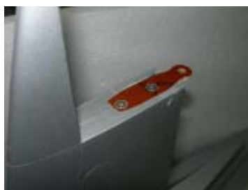
Process of installing the single rudder hinge post. Take great care because this is the only one...
