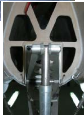
Here you see the springs mounted between the tail gear and the door control horns.
