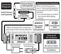
We recommend you add an optional remote antenna when you use this receiver in very demanding environments. For example, where the model is constructed from materials which shield RF (such as carbon fiber).
