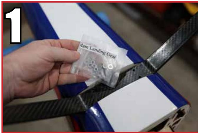
Attach the landing gear to the fuselage using the 4mm screws, washers and nyloc nuts. You will need to use pliers to hold the nyloc nuts inside the fuselage as you tighten the screws.
