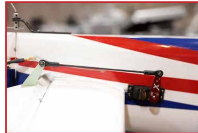
Apply epoxy glue to the rudder horn where it will be inside the slot in the rudder. Press the horn into the rudder until it is centered. Assemble the ball link and screw on the opposite side, make certain the horn assembly is centered, and add the square horn plates with epoxy as shown. Clean up any excess epoxy with alcohol and allow to cure.
