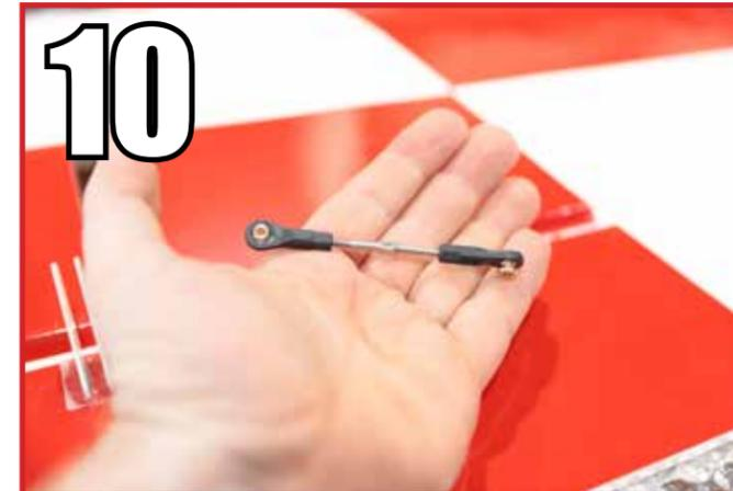
The aileron hinges and horns are installed in exactly the same manner as the elevator and rudder hinges and horns. Once this is completed, assemble the aileron pushrods as shown. Note that these are threaded one right hand, one left hand. This allows them to be adjusted without removal from the aircraft.
