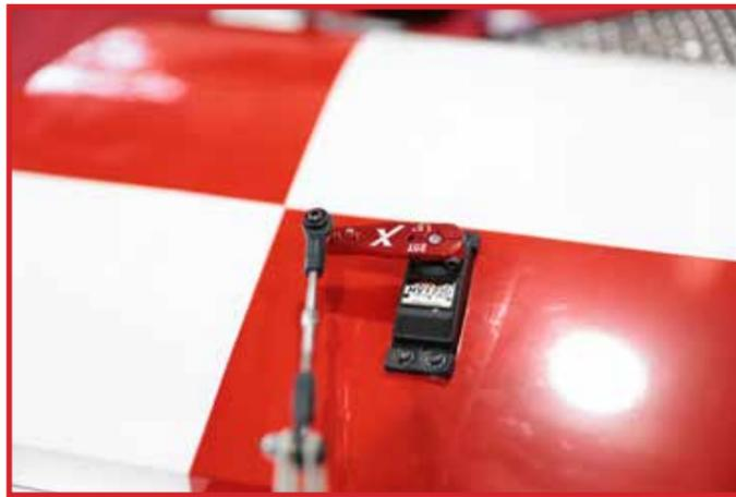
We recommend Extreme Flight RC 1.5" aluminum servo arms for the ailerons. Adjust the pushrod length by rotating them with using the nut in the center of the pushrod.
