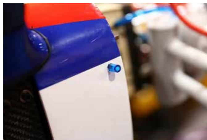
Measure the location of the exhaust outlets from the firewall. Transfer this dimension to the bottom of the cowl and cut the required openings. We use a Dremel tool for this job - protect your eyes and lungs from dust.
