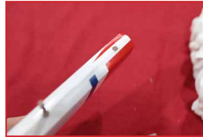
When you press the hinges into the hinge holes, some epoxy may squeeze out. Use alcohol on a rag to clean up any excess epoxy.
