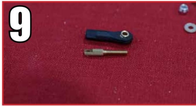
The rudder connection is by pull-pull cable. The ends of the cables are made by screwing the brass cable ends into the nylon ball links.
