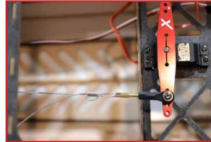
Cross the cable across each other inside the fuselage to form an X shape. Install your rudder servo and arm as shown. Pictured is the Extreme Flight RC 4" aluminum arm, our recommendation. Install the front cable ends and attach to servo arm, as shown. Screw the cable ends farther into the ball links to tighten the cables. Cut off excess cable, leaving 1/2" (12mm) end from the crimps.
