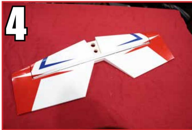
Locate the horizontal stabilizer and elevators. In this step we will hinge the elevators, and we will hinge all the other surfaces in the same manner. Note that for hinging, we will be using 30 minute spoxy for adhesive, and denatured alcohol and a rag for cleanup.
