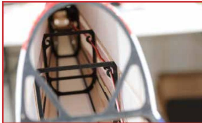
Test fit your horizontal stabilizer assembly into the fuselage. Check for fit. Note how much force it takes to slide the stab all the way forward into the slot until it contacts the front of the cutout. Make sure your stab is *correct side up*.
