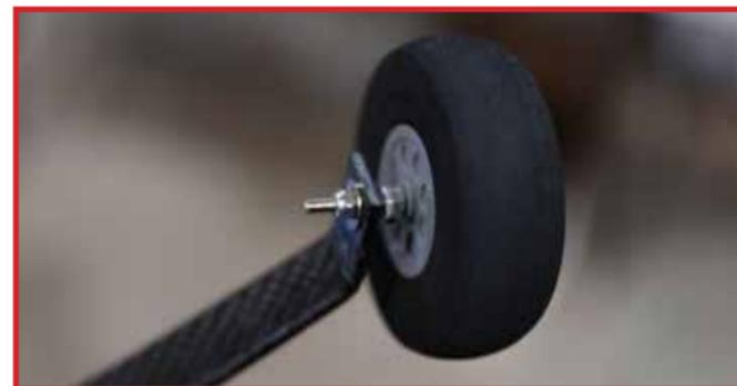
Slide wheel collars onto the axles, then the main wheels, then outer wheel collars. The wheel collars locate the wheels on the axles, when you install the pants you will need to fine-tune the location of the wheels. Apply a drop of loctite to the set screws in the wheel collars and tighten them.
