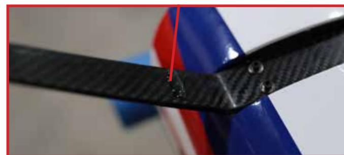
Place a large dollop of goo-adhesive onto the gear leg as shown, then slide the fairings into the gear legs. The Goo will fill up the end of the fairings. Place an additional dollop of Goo where the fairings contact the fuselage. Allow the Goo to dry while you install the wheels and wheel pants.
