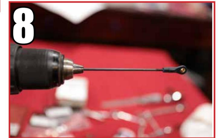
Install the servo arm and pushrod. We recommend Extreme Flight RC aluminum servo arms. Pictured is a 1.5" arm, but we recommend a 2.0" arm for maximum options in control throw. Install the pushrod with 3mm hardware, note that you must use either a nyloc nut or loctite on the screw which attaches the ball link to the servo arm.
