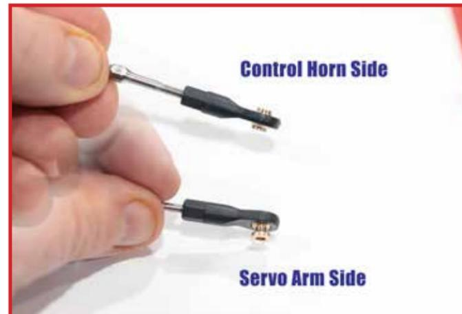
Note that the 74" Slick 580 EXP uses two different types of ball joints. One is symmetrical and is used on the fiberglass control horns in the surfaces. The other is asymmetrical, with a raised pedestal on one side, and it is used on the servo arms.
