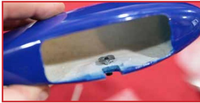
Increase the drill size until you can press the blind nut into the hole as shown. Use the 3mm screw and washer to draw the blind nut into the hole part way and the spikes on the blind nut engage the fiberglass.
