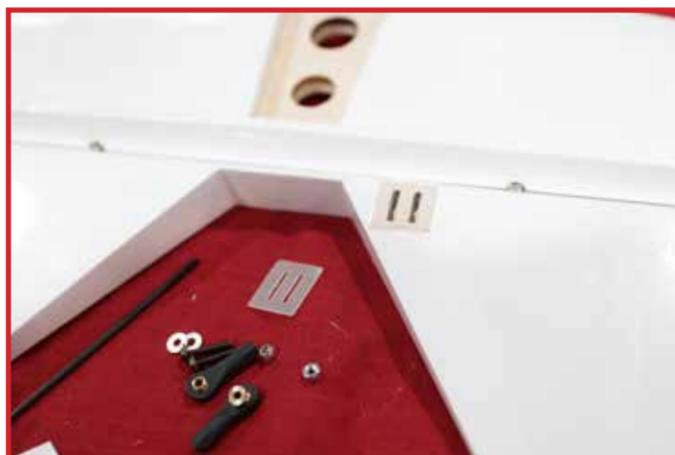
Use sandpaper or an emery file to roughen the part of the control horn which will be inserted into the elevator. We do this to ensure the best possible glue joint on this super-critical connection.
