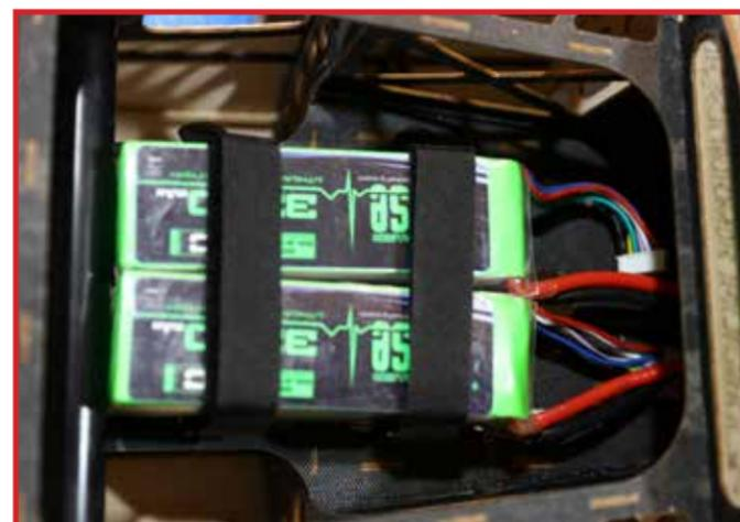
For electric power, use strong velcro straps to restrain the lipo battery packs as shown.
