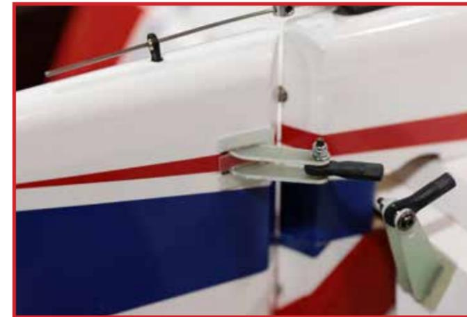
Locate the elevator pushrod, and remove the ball link from the elevator horn. To assemble the elevator pushrod, you will need to screw the ball links onto the elevator pushrod. We prefer to use a cordless drill. Chuck the bare pushrod in and hold the first ball link, and screw in as shown. Then, we turn the shaft around, and chuck the ball link into the drill to install the second ball link. NOTE: both ends of the elevator pushrod are conventional "right hand" threads.
