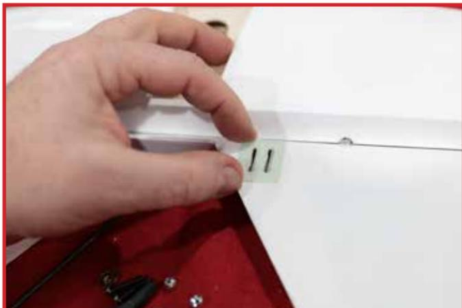
If necessary, clean out the slots in the elevator of any stray wood fibers so the control horn can easily be inserted.
