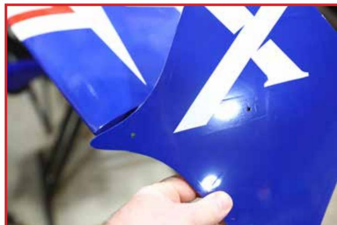
Screw on the wingtips and SFG's on as shown. Because these parts need to be removed for transporting the aircraft, do not loctite these screws.
