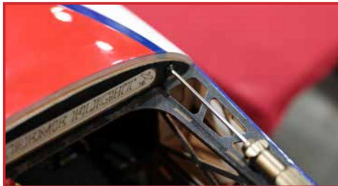
Install the cowling by sliding it up onto the lower hooks, from the bottom, and installing the two cowl screws as shown.
