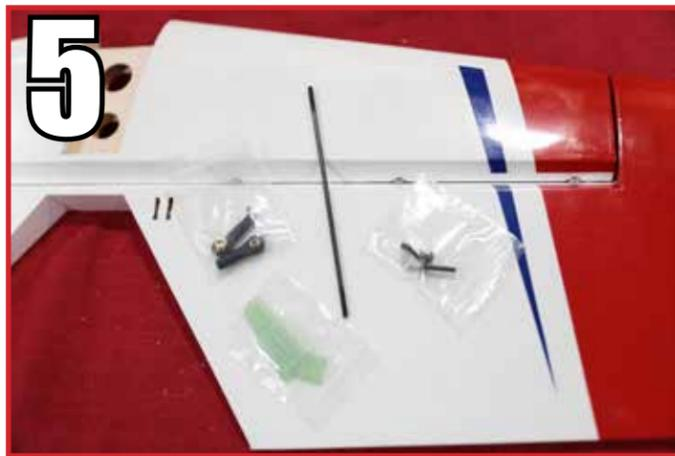
Once the hinges are cured, locate the hardware for the elevator as shown. We will be installing the control horn, and we will install all remaining horns using this procedure.
