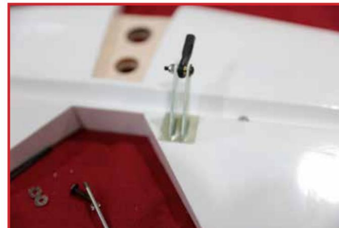
Place the baseplate on the horn as shown, mix a new batch of 30 minute epoxy, and coat the baseplate and legs of the horn assembly with epoxy. Place more epoxy into the slots in the elevator and insert the horn assembly. Clean up any excess epoxy which comes out. Allow to cure.
