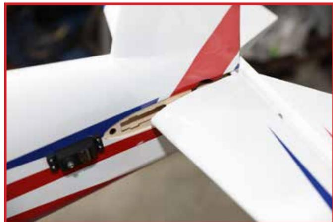
Apply 30 minute epoxy glue to the bare wood area of the stabilizer, top and bottom, and into the slot in the fuselage.
