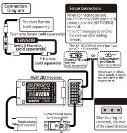
We recommend you add an optional remote antenna when you use this receiver in very demanding environments. For example, where the model is constructed from materials which shield RF (such as carbon fiber).
