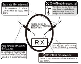
This receiver features antenna diversity. It is extremely important to position the antenna correctly. Be sure to read the above explanation and follow these instructions.
