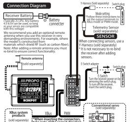
\* When using the XBus system, the transmitter must be set to XBus mode A and programmed to control the applicable XBus products
