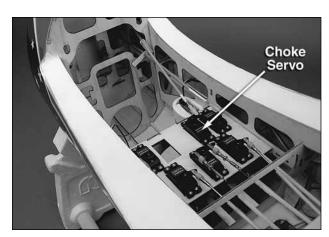
☐ 9. Install the servo operated choke following the same procedure.
