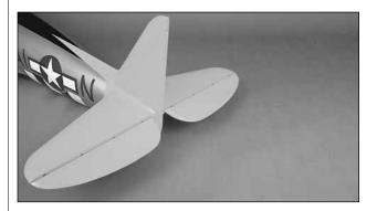
☐ 3. Gather everything required for gluing the stabilizer halves to the fuselage, including 30-minute
