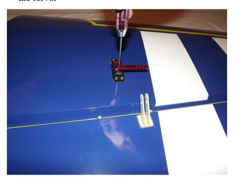
26. Use the recommend 1.5" SWB servo arms and attach 2 ball links onto the titanium turnbuckle pushrod. Secure the pushrod to the control horns and servo arm using the supplied 3mm bolts, washers, and nylon insert locknuts as shown in the picture below. As always, use blue Loctite on ALL bolts!
