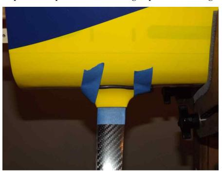
45. Once the silicon glue has thoroughly cured, remove the blue painters tape and clean up any residual glue using denatured alcohol.
