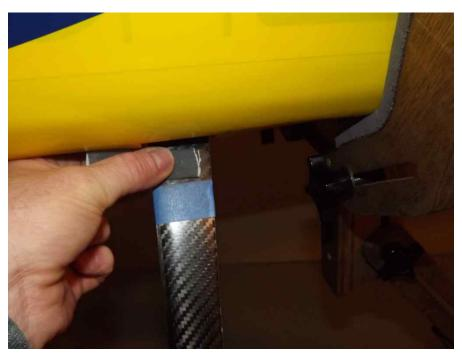
44. Secure the fairing to the gear with "Goop" silicon glue and use additional blue painters tape to hold the fairing in place while the glue dries.
