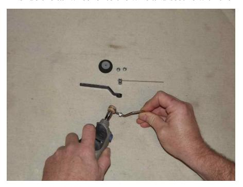
35. Use a sharp hobby knife to open the 3 holes in the bottom rear of the fuselage to expose the 3 pre-installed 3mm blind nuts. Slide the tiller arm of the tailwheel into the hole in the ball link and attach the tailwheel assembly to the bottom of the fuselage with the 3 medium length 3mm bolts and washers. Be sure to apply blue Loctite to ALL bolts!
