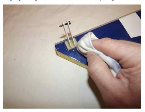
10. Next, remove the pin hinges from the horizontal stabs.
