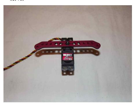
38. Install the rudder servo using the supplied hardware with the output shaft toward the front of the plane.
