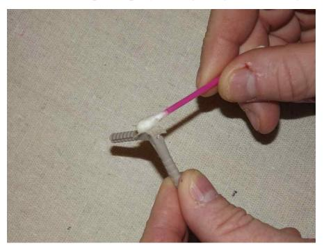
12. Mix a generous batch of 30 minute epoxy. Use a zip tie or an old pushrod to thoroughly coat and fill the hinge holes on the stab with epoxy.
