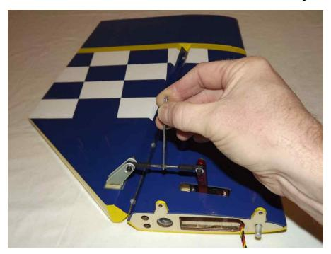
22. Set the servo endpoints to achieve maximum travel. You may need to enlarge the size of the servo arm exit slot. Repeat these steps for the other stab assembly.
