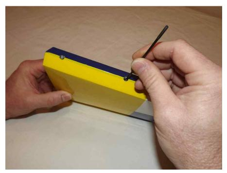
13. Next, coat one side of all 4 hinges with epoxy and push the hinges into the holes of the horizontal stab.
