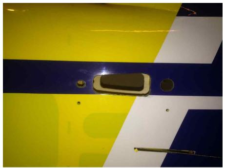
61. Attach 36 inch servo extensions to each elevator servo. If you plan to remove the stabs for transport, you will need 48 inch extensions. Slide the stab halves onto the carbon fiber stab tube and secure with a 3mm bolt and washer inserted through the
