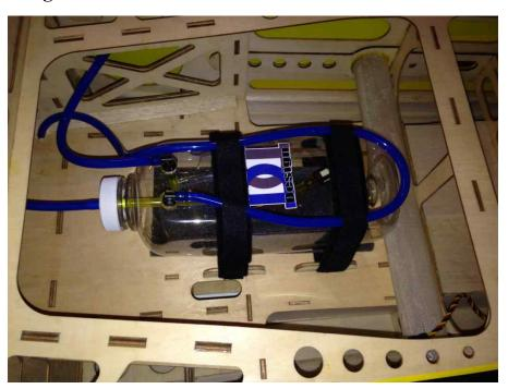
55. Find a location toward the front of the fuse to install a fuel dot. Here is where we installed ours.
