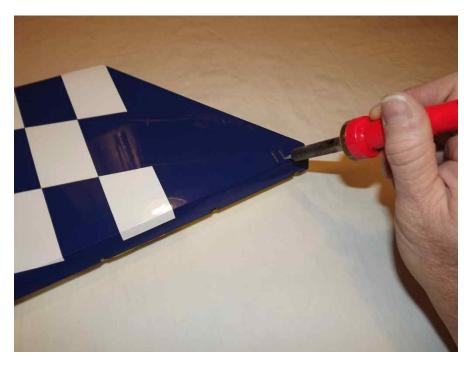
2. Insert the 2 control horns into the base plate and trial fit the horns into the slot, making sure they seat properly against the base and elevator surface.
