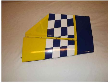
Note: Before installing the servos, it's a good time to seal the hinge gap with a strip of Ultracote or Blenderm tape. Also, I recommend that you thin a small amount of epoxy with a few drops of alcohol and apply a light coat to the inside of the stab and to the servo mounting rib as well as to the root rib and mounting tabs to protect against exhaust residue that can collect in these areas.
