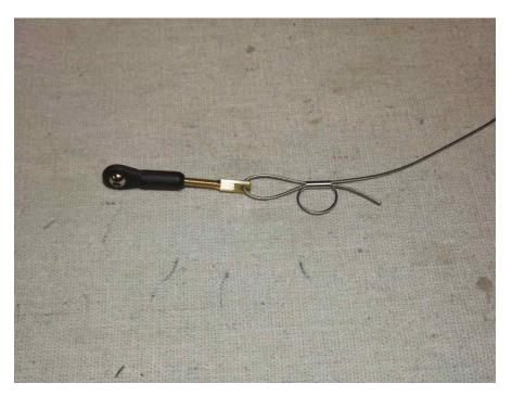
40. Insert the bare end of the cable into the slot in the rear of the fuselage and feed it forward into the canopy area. Make the same type of linkage as done previously. Electronically center the servo and secure the linkage at both ends with a 3mm bolt and nylon insert lock nut. Repeat for the other side.
