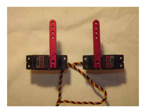
18. Using the manufacturer supplied mounting hardware, install the elevator servo with the output shaft toward the rear of the stab and re-attach the servo arm.
