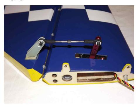
21. With the servo arm centered (as described in Step 17), adjust the turnbuckle on the control rod until the elevator is in the neutral position.
