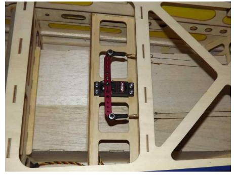
Note: When routing the pull-pull cables through the fuse, they should cross like an "X". Also, the tension on the wires should be taut but not overly tightened.
