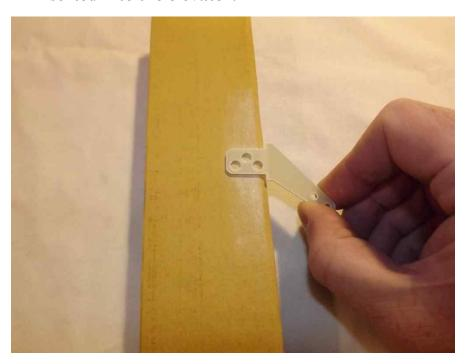
7. Apply 30 minute epoxy to the elevator slots using a zip tie to ensure the slots are filled will epoxy.
