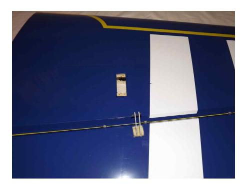
25. Attach a 12" servo extension to your servo and secure with thread or heat shrink tubing. Use the manufacturer supplied mounting hardware to install the servo with the output shaft toward the trailing edge of the wing. Electronically center the servo.
