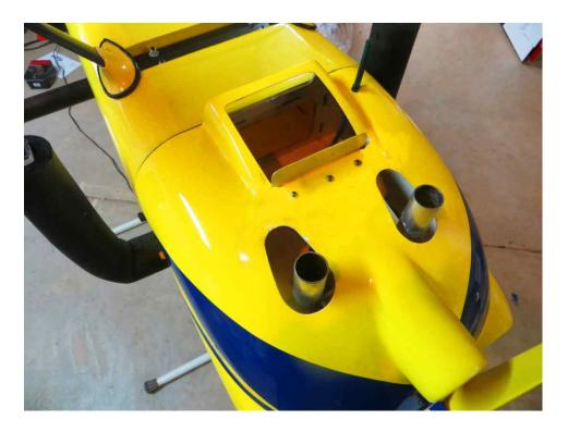
59. Once you're satisfied with the fit of the cowl, add some thick CA or Epoxy to the intersection of the cowl and plywood cowl ring. Slide the cowl into position and secure with 4 x 3mm bolts and washers through the pre-drilled holes in the cowl.
