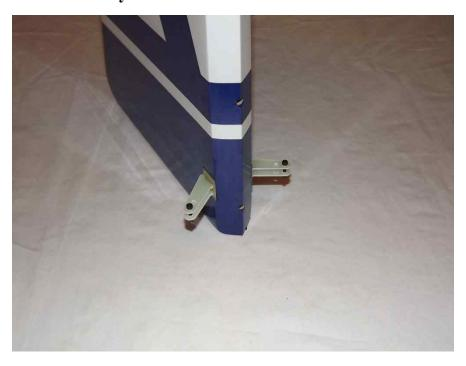
32. Locate a 2mm ball link from the hardware bag. Measure 3" back from the leading edge of the rudder and drill a 3/16" hole to accept the shank on the ball link. Scuff the shaft of the ball link and glue the ball link into the hole as shown below.
