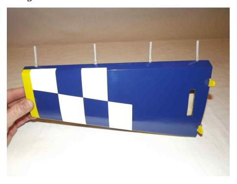
15. Now coat the other side of the hinges as well as the hinge holes in the elevator with epoxy and install the elevator onto the stab. Don't forget to apply epoxy in the hinge holes on the stab before installing the stab to the elevator.
