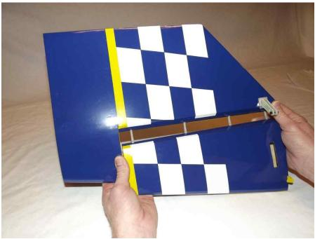
16. Use denatured alcohol and a cloth to remove all excess epoxy, especially on the hinge pin. Make sure you have full deflection in both directions — once satisfied with the results, set the surface aside to dry. After the hinges have dried thoroughly, pull on them to make sure they are properly installed.
