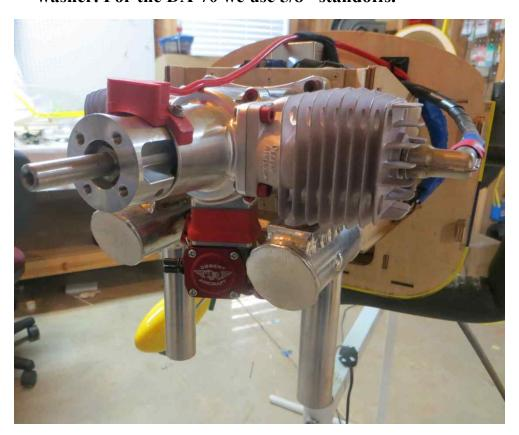
52. Next, install the throttle servo in the pre-cut servo hole located in the bottom of the motor box. Locate the 2mm pushrod and white ball links to fabricate the throttle linkage. If using a pipe you will need to add 3/8" hardwood rails to raise the servo.
