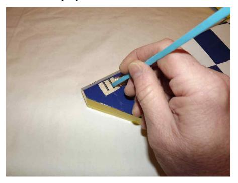
8. Also, apply a generous amount of epoxy to the bottom of the G-10 control horns and base plate.
