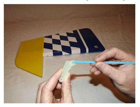
31. Install the rudder horns and base plates into the rudder one side at a time. Clean any excess epoxy from the rudder, recheck the alignment and set the assembly aside to dry.
