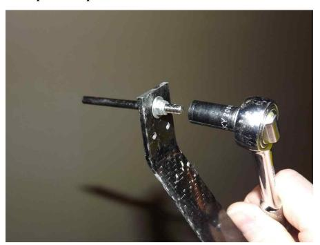
47. Install one wheel collar on the axel first in order to center the wheel in the wheel pant. Next, slide the wheel onto the axel and secure the wheel with the second wheel collar. Repeat this process for the remaining wheel.
