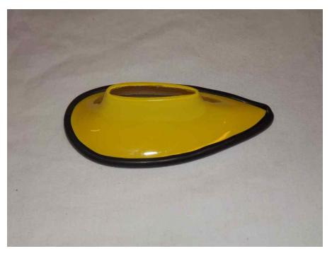
43. Temporarily slide the fairing onto the gear and up against the fuselage. Place some blue painters tape at the bottom of the fairing to mark the location on the gear. Lightly sand the gear leg where the fairing will attach.
