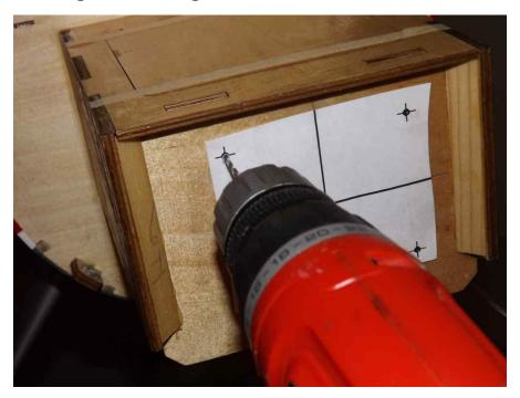
51. Use the recommended mounting bolts to mount the engine to the firewall making sure to use large washers behind the firewall to distribute the load. Use standoffs to ensure the motor extends 6 5/16 inches from the firewall to the engine thrust washer. For the DA-70 we use 5/8" standoffs.
