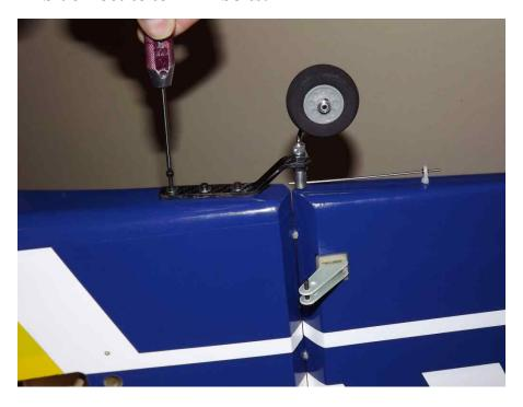
36. Next, install the pull-pull rudder cables. First remove the covering from the exit slots at the rear of the fuselage as shown below.
