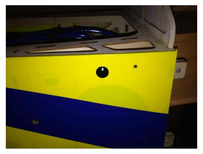
56. Once the throttle linkage is installed and all the plumbing is completed, install the engine box cover with 4 wood screws. You may want to take the time to install some blind nuts and use bolts for this.
