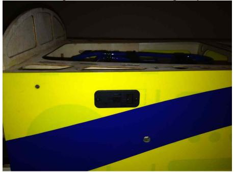
58. Slide the cowl into position and align the 4 slots in the cowl ring with the mounting tabs in the fuse. Cut the cowl to clear the muffler and spark plug wire. Also it's a good idea to cut an opening in the bottom of the cowl for an air exit to allow for proper cooling.
