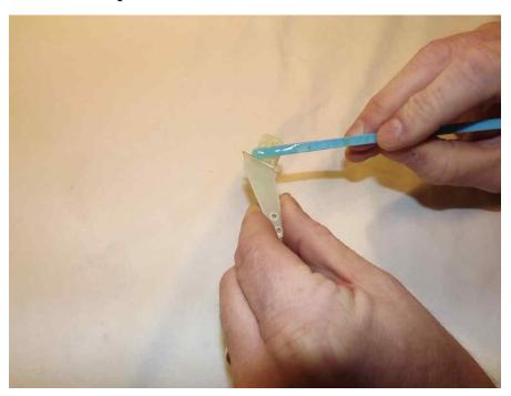
9. Reinsert the assembly into the elevator and wipe away any excess epoxy with a cloth and denatured alcohol. Place a 3mm bolt through the horns to help insure proper alignment and set aside to dry. Repeat for the other elevator half.
