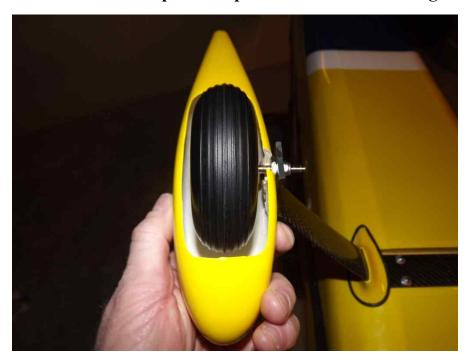
48. Install the wheel pant using the supplied 3mm bolts and washers as shown in the picture below. As always, use blue Loctite on ALL bolts! Repeat this process for the remaining wheel pant.
