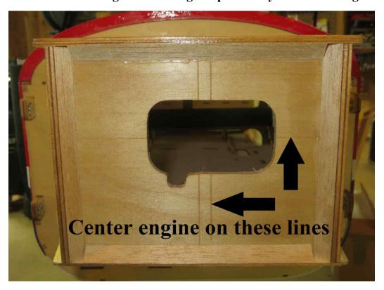
50. Tape the engine manufacturers mounting template onto the front of the firewall making sure to align the horizontal and vertical lines on the template with the laser scribed lines on the firewall. Be sure to use the offset line to the right of the vertical center line in order to accommodate for the motor offset due to the built in right thrust angle in the motor box.
