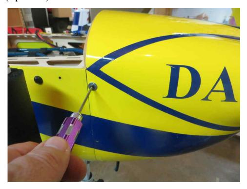
60. Before installing the stab/elevators, remove the covering in rear sides of the fuse to expose the pre-mounted 3mm blind nuts. You will also need to open a hole for the servo leads to pass through.
