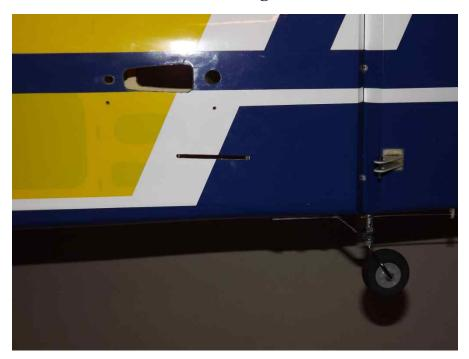
37. Locate the rudder servo and install the recommended SWB 4" offset rudder arm as shown in the picture below. Also it's a good time to electronically center the servo.
